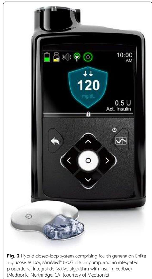
**Fig. 2** Hybrid closed-loop system comprising fourth generation Enlite 3 glucose sensor, MiniMed® 670G insulin pump, and an integrated proportional-integral-derivative algorithm with insulin feedback (Medtronic, Northridge, CA) (courtesy of Medtronic)
